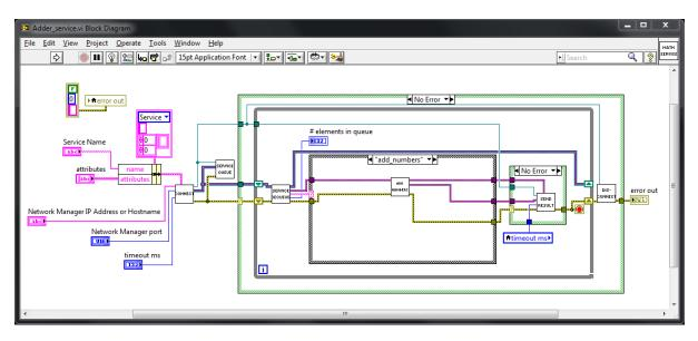
Run Adder\_service.vi to start the *Adder* Service and then on another computer you can send a request to the *Adder* Service
